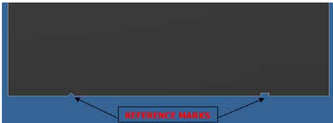
Figure 3 – Illustrative drawing of reference marks on the mask
