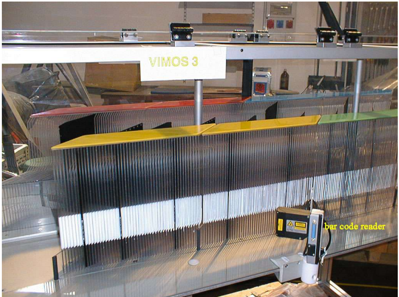
Figure 2 : Close-up view of the VIMOS Storage Cabinet and bar code reader
