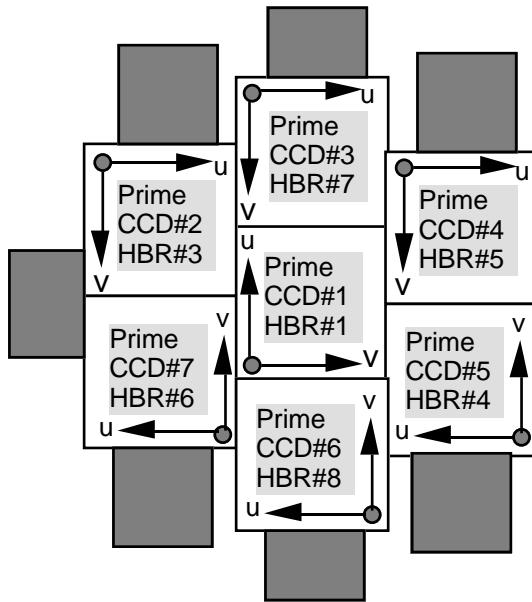
The  $u_i, v_i$  node detector coordinates are in pixel. The  $u$  coordinate ranges 0 to 609, as it includes two extra regions of 5 pixels on both sides for overscan. The  $v$  coordinate ranges 0 to 601, as it includes an extra region of 2 pixels on top.
