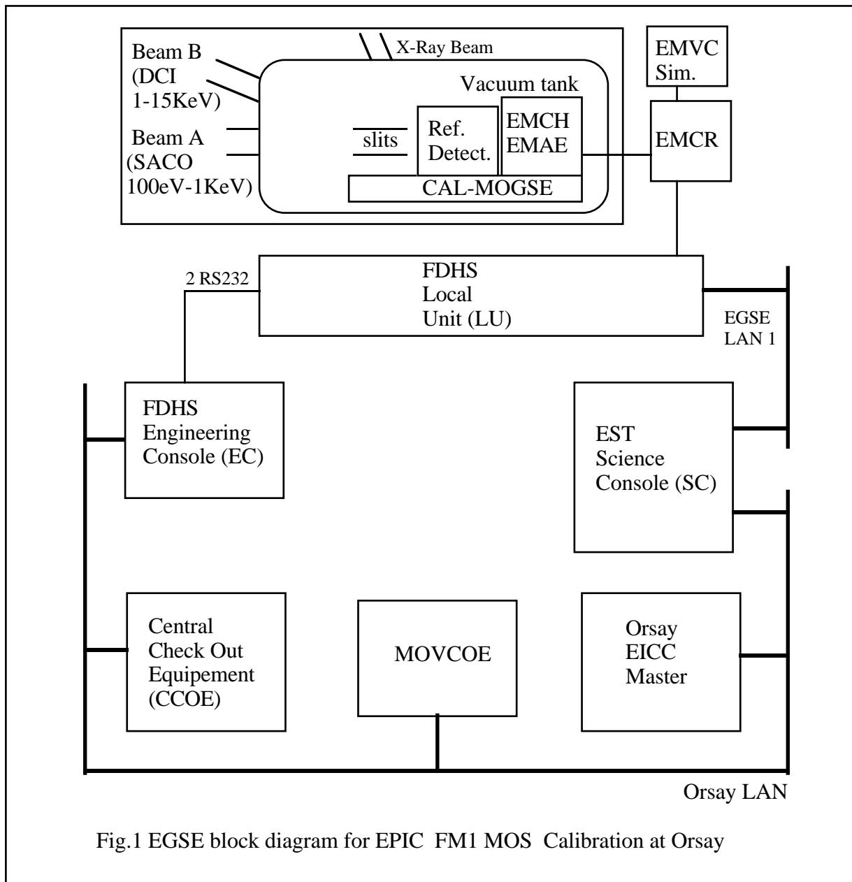
The tests have been conducted from the Central Cechout Equipment (CCOE) which sequenced the operations by means of automated test sequences, implemented as specified in [4] and [5].
