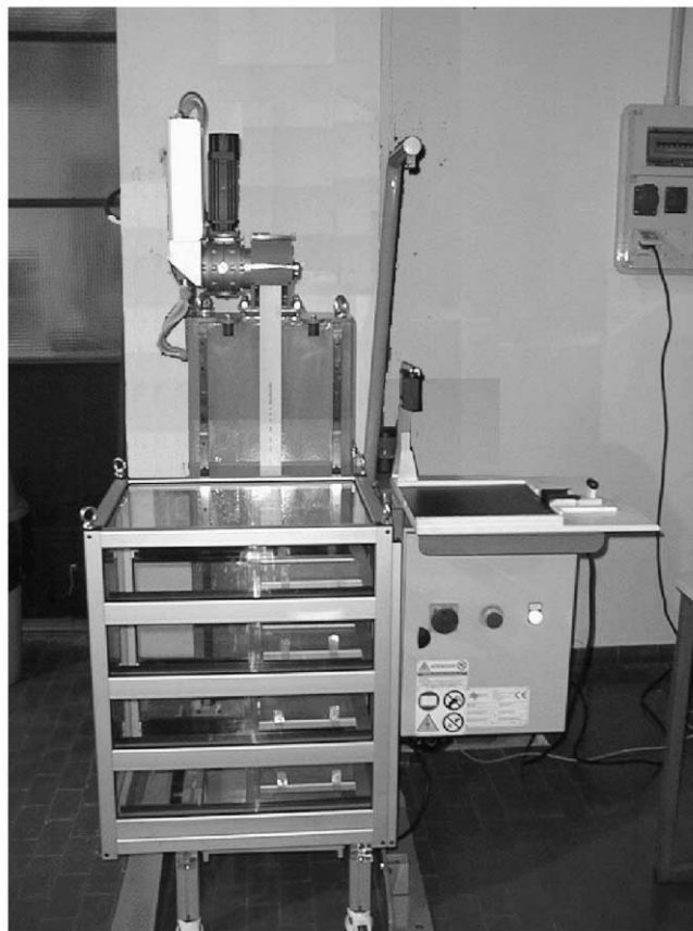
FIG. 5.—The VIMOS instrument cabinet robot with the empty IC box placed on its platform and a mask positioned on the stand.
