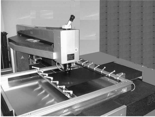
FIG. 2.—LPKF laser cutting machine installed in Milano. An invar sheet is mounted and clamped on the working platform. For mask cutting, the laser focusing system moves down close to the sheet and the whole platform is displaced in the X and Y directions.
